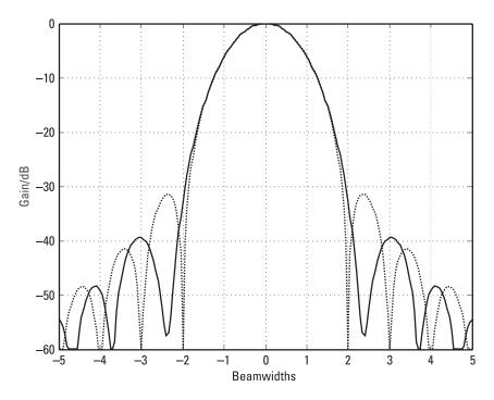
Figure 7.4 Beam pattern for ULA with additional shading.
