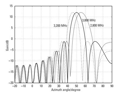
Figure 6.6 Array response with narrowband weights.
