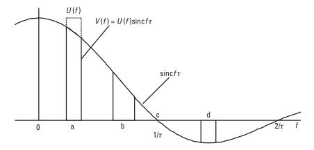
Figure 4.16 Spectrum of waveform sampled with a finite window.
