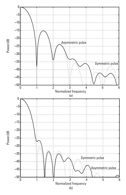
**Figure 3.8** Asymmetric trapezoidal pulse spectra: (a) edges 0.2T and 0.3T; and (b) edges 0.6T and 0.8T.
