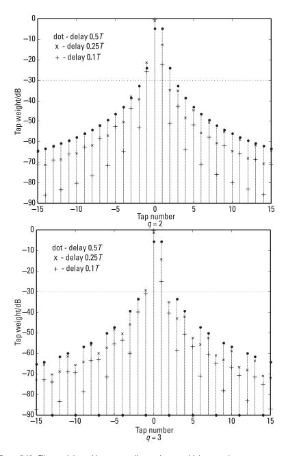
Figure 5.10 Filter weights with oversampling and trapezoidal spectral gate.
