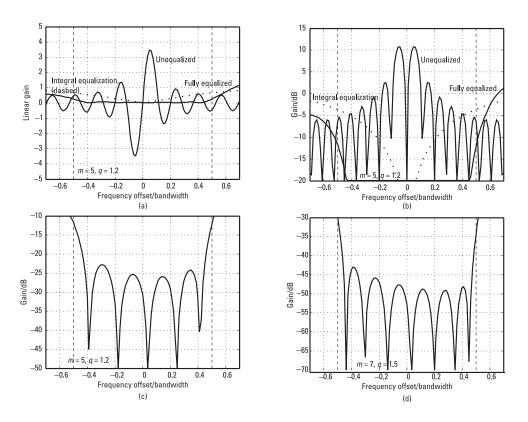
Figure 6.15 Difference beam gain response against frequency offset: (a) linear response; (b) logarithmic response; (c) expanded equalized response; (d) response with more processing.
