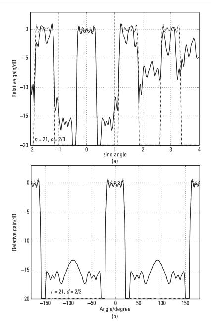
**Figure 7.10** Sector pattern from an irregular linear array: (a) response in u-space; (b) beam pattern.
