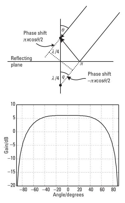
Figure 7.7 Element response with reflector.
