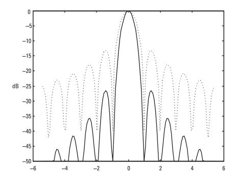
Figure 3.5 Spectrum of triangular pulse.
