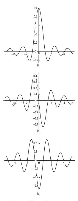
Figure 6.3 First three snc functions: (a)  $snc_0$ ; (b) $snc_1$ ; and (c)  $snc_2$ .
