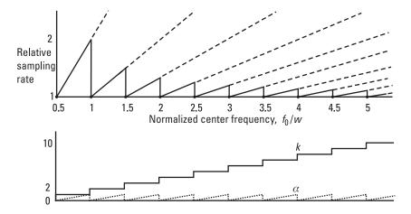
Figure 4.11 Relative sampling rates (basic quadrature sampling).
