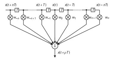
Figure 5.16 FIR filter for interpolation.
