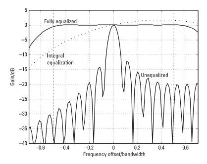
Figure 6.18 Sum beam gain with frequency sensitive elements.
