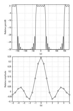
Figure 7.6 Sixty-degree sector beam from an array of 21 elements: (a) beam pattern; (b) element weights.
