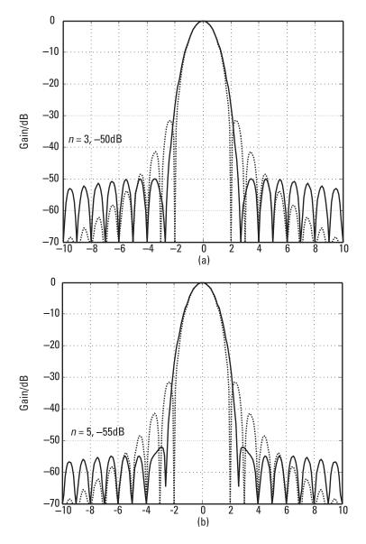
Figure 7.5 Constant-level side-lobe patterns: (a) first two lobes nominally at -50 dB; and (b) first four lobes nominally at -55 dB.
