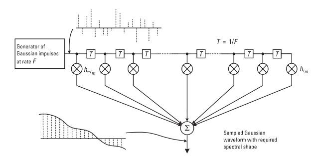
Figure 5.19 FIR filter for Gaussian waveform generation.
