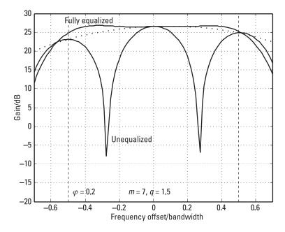
Figure 6.17 Difference beam slope, 20% bandwidth.
