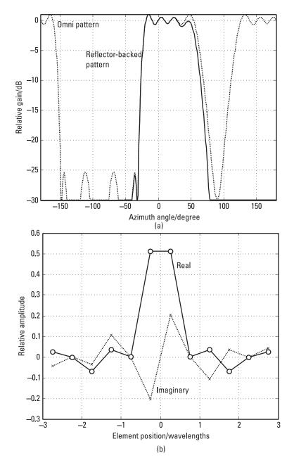
Figure 7.8 Steered sector beam with reflector-backed elements: (a) beam patterns; (b) element weights.
