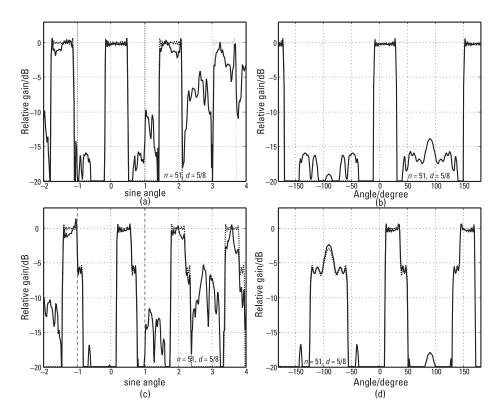
Figure 7.11 Sector patterns from a steered irregular linear array: (a) response in u-space, beam at 10 degrees; (b) beam pattern, beam at  $10^{\circ}$ ; (c) response in u-space, beam at  $30^{\circ}$ ; (d) beam pattern, beam at  $30^{\circ}$ .
