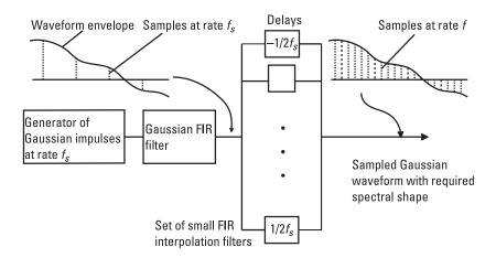
Figure 5.20 Gaussian waveform generation with interpolation.
