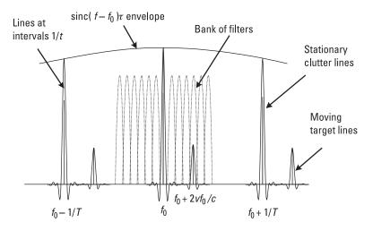
Figure 3.21 Spectrum of pulse Doppler radar waveform.
