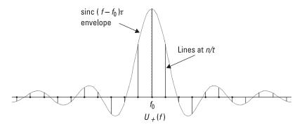
Figure 3.18 Spectrum of regular RF pulse train.
