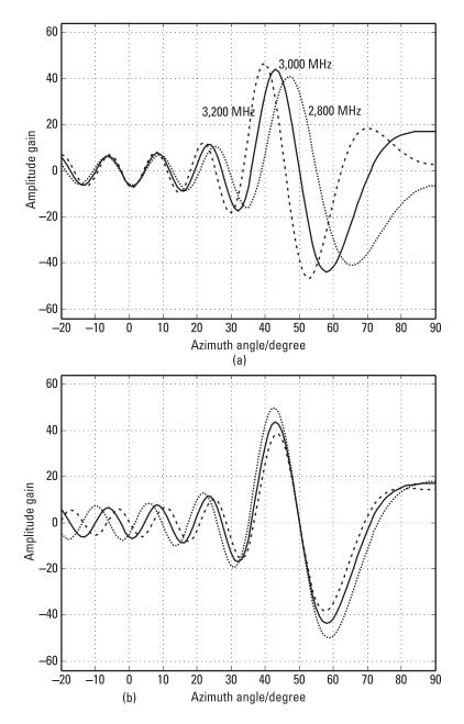
Figure 6.14 Difference beam response: (a) difference beam with narrowband weights; (b) difference beam with equalization.
