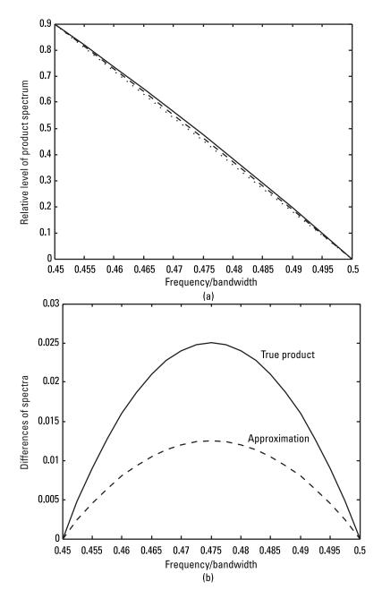
Figure 6.12 Effect of approximation of product spectrum on falling edge of trapezoid: (a) falling edge of product spectra; (b) differences of spectra.
