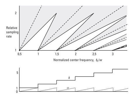
Figure 4.14 Relative sampling rates (modified quadrature sampling).
