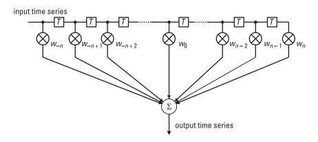
Figure 5.1 FIR filter for interpolation.
