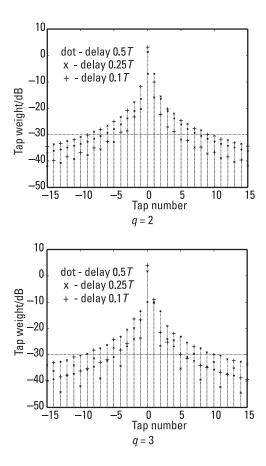
Figure 5.8 FIR interpolation weights with oversampling.
