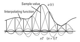
Figure 4.2 Sampled waveform with interpolating functions.
