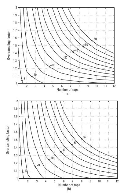
**Figure 5.17** Mismatch powers for two power spectra: (a) rectangular spectrum, and (b) raised cosine spectrum.
