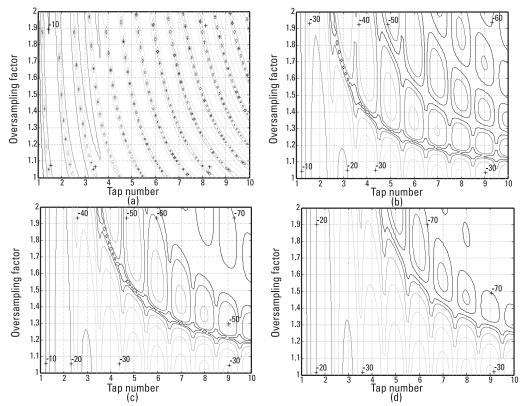
Figure 5.15 Tap weight variation with oversampling rate for four spectral gating functions at delay 0.57: (a) rectangular, (b) trapezoidal, (c) trapezoidal rounded, and (d) raised cosine rounded.
