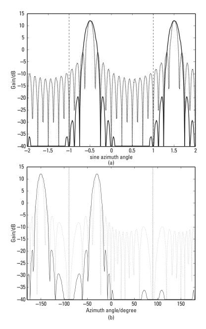
Figure 7.3 Beam patterns for uniform linear array with raised cosine shading: (a) u-space; (b) angle space.
