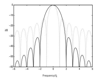
Figure 3.10 Raised cosine pulse spectrum, log scale.
