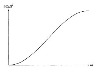
Figure 6.9: The (squared) frequency response of a finite difference filter. With these coefficients the lower frequency components are passed essentially unattenuated, while the higher components are strongly attenuated.
