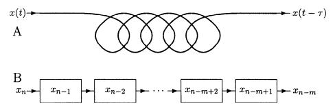
Figure 6.3: Implementation of the simple delay. In (A) we see how an analog delay of lag  $\tau$  can be obtained by allowing a voltage of current signal to travel at finite velocity through a sufficiently long delay line. In (B) a digital delay of lag m is implemented using a FIFO buffer.
