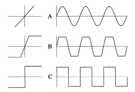
Figure 6.1: The effect of clipping amplifiers with different gains on sinusoidal signals. In (A) there is no clipping, in (B) intermediate gain and clipping, while (C) represents the infinite gain case (hard limiter).
