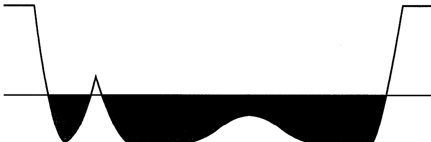
Figure 18.11: The water pouring criterion states that the information rate is maximized when the amount of power available to be transmitted is distributed in a channel in the same way as water fills an irregularly shaped bowl.
