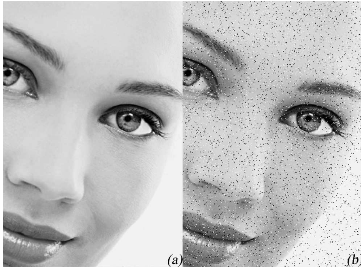
Figure 20: (a) Original image, (b) Image with 5% salt-and-pepper noise (PSNR=17.75dB)
