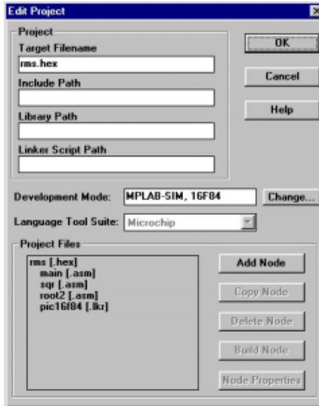
Fig. 8.6 MPLAB window showing files selected to assemble, link and simulate Program 8.4.
