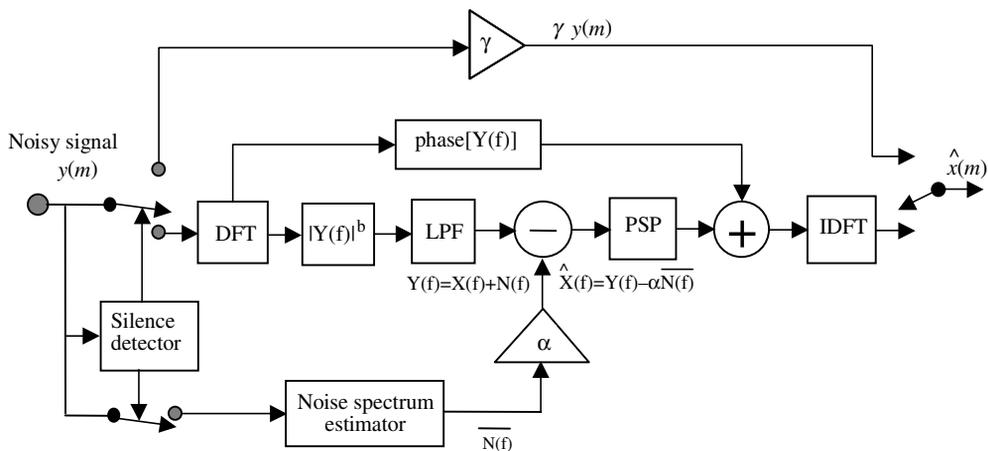
**Figure 11.7** Block diagram configuration of a spectral subtraction system.
