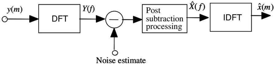
**Figure 11.2** A block diagram illustration of spectral subtraction.
