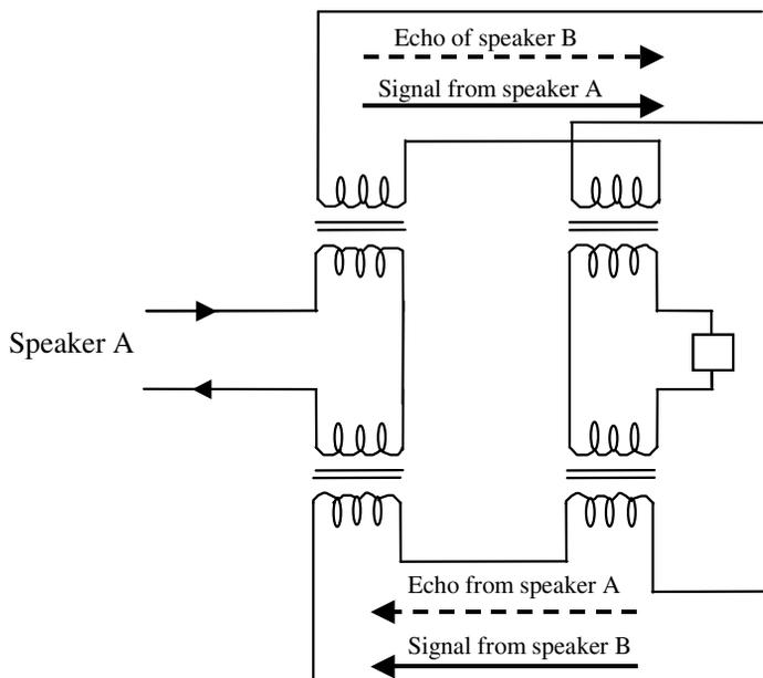
**Figure 14.3** A 2-wire to 4-wire hybrid circuit.
