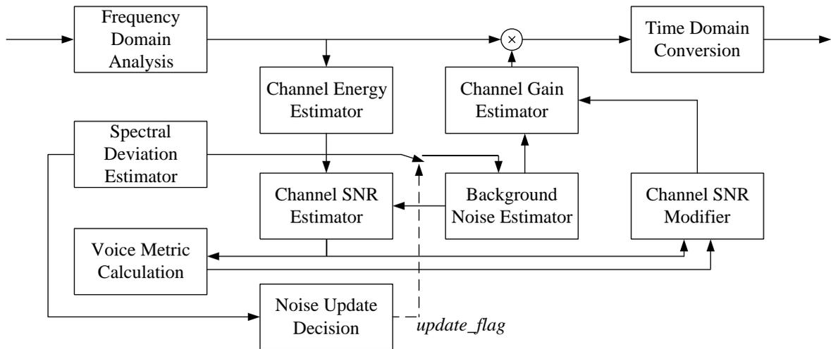
**Fig. 2.3** EVRC Noise Suppression Block, redrawn from [21].
