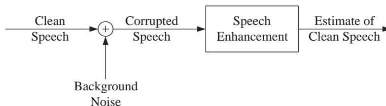
**Fig. 1.3** Block diagram of basic speech enhancement.
