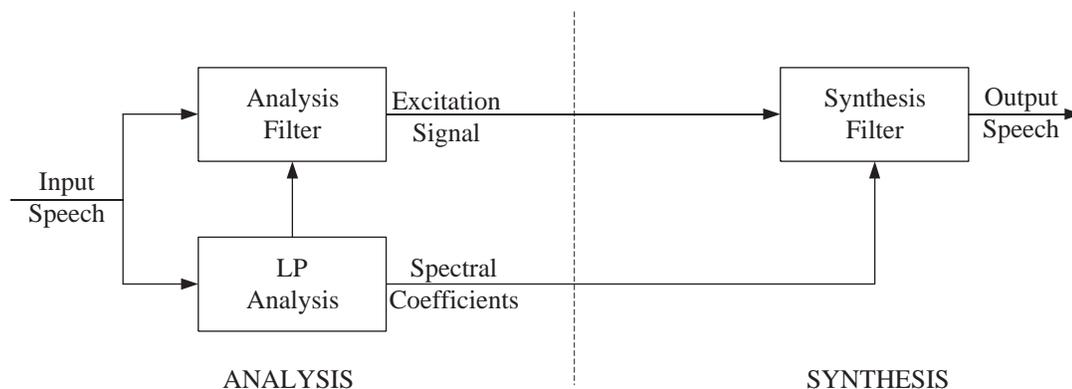
**Fig. 1.1** Block diagram of a basic vocoder
