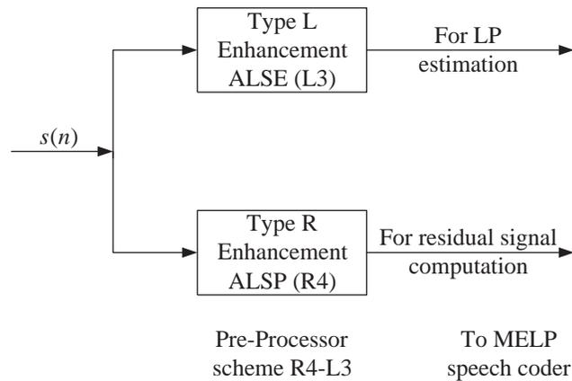
**Fig. 4.1** Basic system under test.
