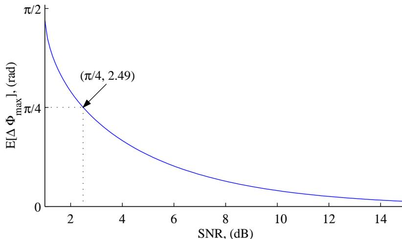
**Fig. 2.11** Expected maximum phase error vs. input Signal-to-Noise-Ratio.
