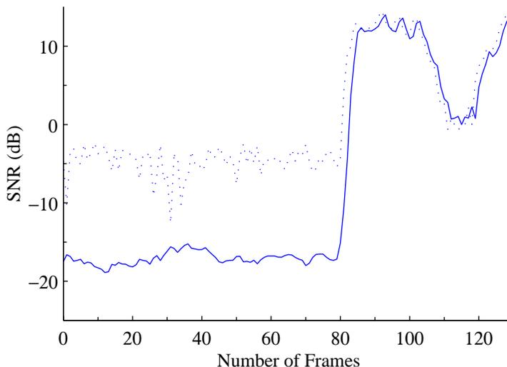
**Fig. 2.10** SNR in successive short-time frames. Dotted: *a posteriori* SNR,  $\gamma_k$ ; Solid: *a priori* SNR,  $\xi_k$ . For the first 80 frames the analyzed signal is pure noise. For the next 50 frames an analyzed signal of 20 dB SNR emerges.
