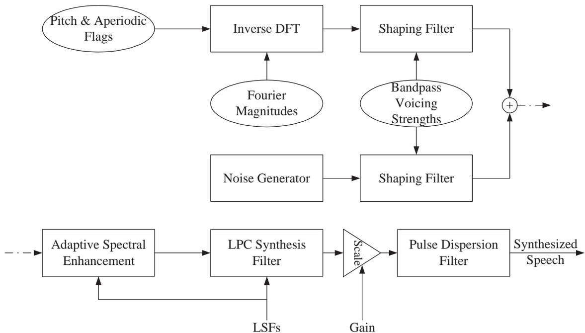
Fig. 3.1 MELP decoder block diagram. Redrawn from [40].
