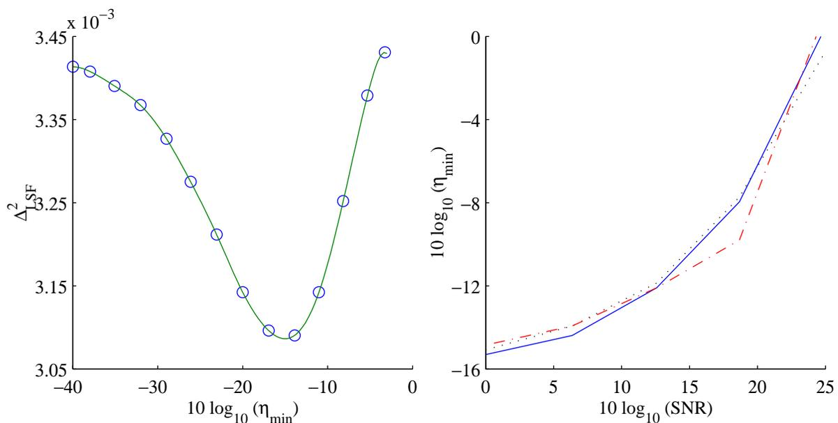
(a) LSF distortion measure  $\Delta_{LSF}^2$  vs.  $10 \log_{10}(\eta_{min})$  for input female speech with 0 dB SNR. Redrawn from [45].
