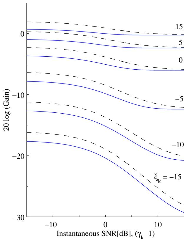
**Fig. 2.8** Parametric gain curves describing  $G_{\text{MMSE}}(\xi_k, \gamma_k)$  defined by Eq. (2.15) (solid) and  $G_{\text{LSA}}$  defined by Eq. (2.33) (dashed) for various values of  $\xi_k$  (in dB).
