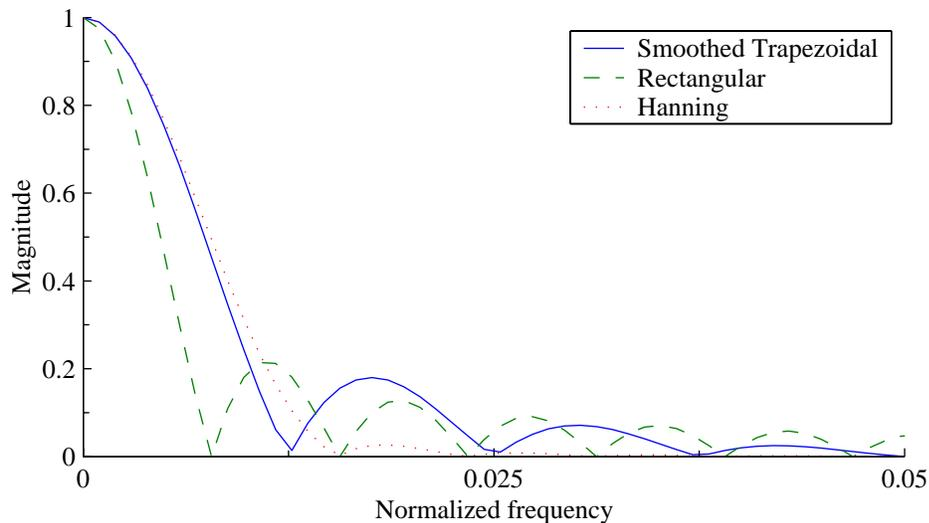
**Fig. 2.2** Frequency Response for three symmetric windows. Solid: smoothed Trapezoidal; Dashed: Rectangular; and Dotted: Hanning Window.
