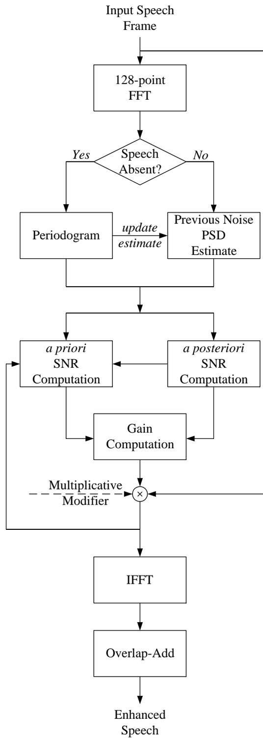
**Fig. 2.4** Algorithm for MMSE-STSA.
