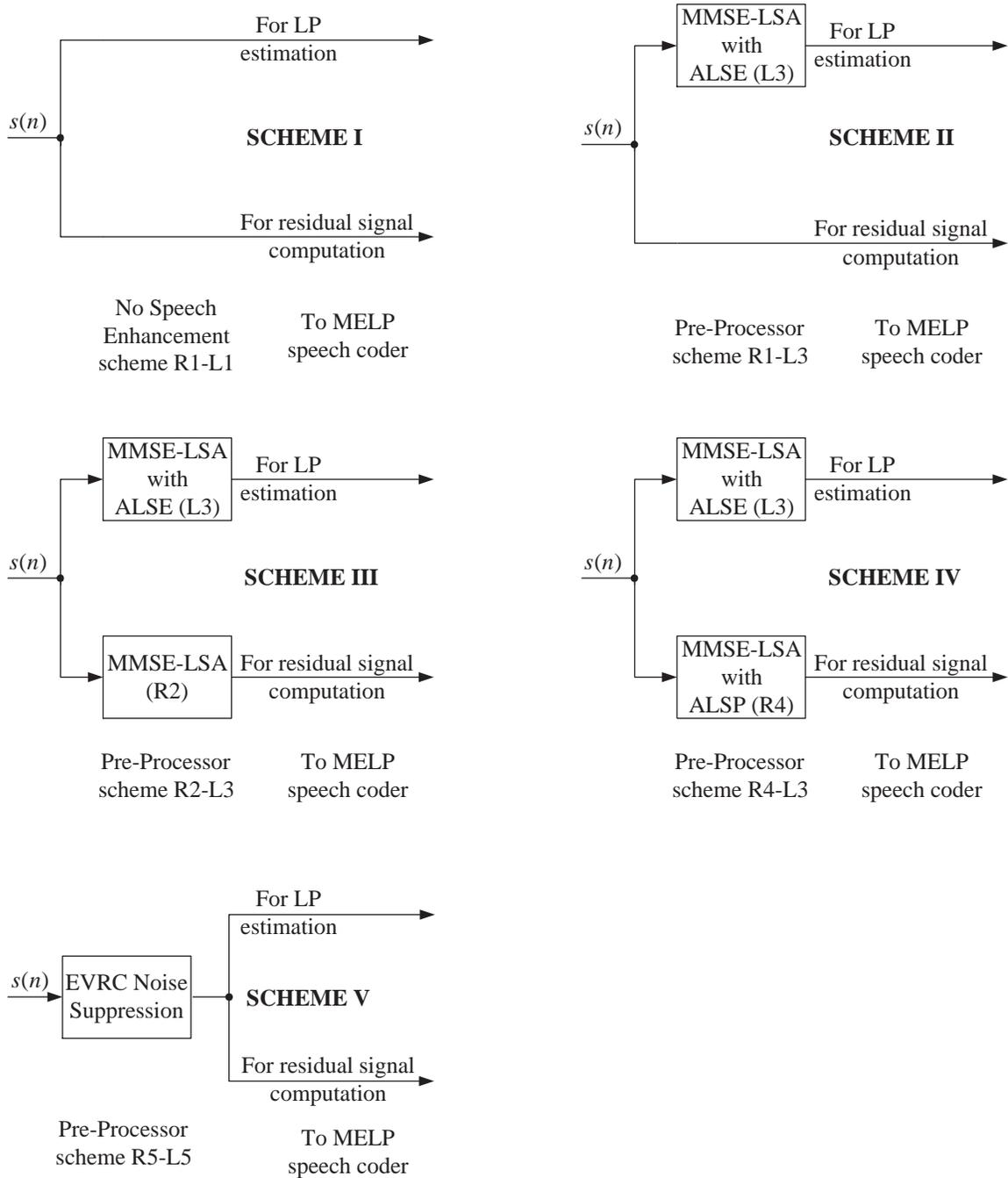
Fig. 4.2 Schemes on which the A-B was conducted.
