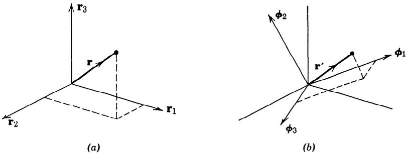
Fig. 2.33 Coordinate systems: [a] original coordinate system; [b] new coordinate system.
