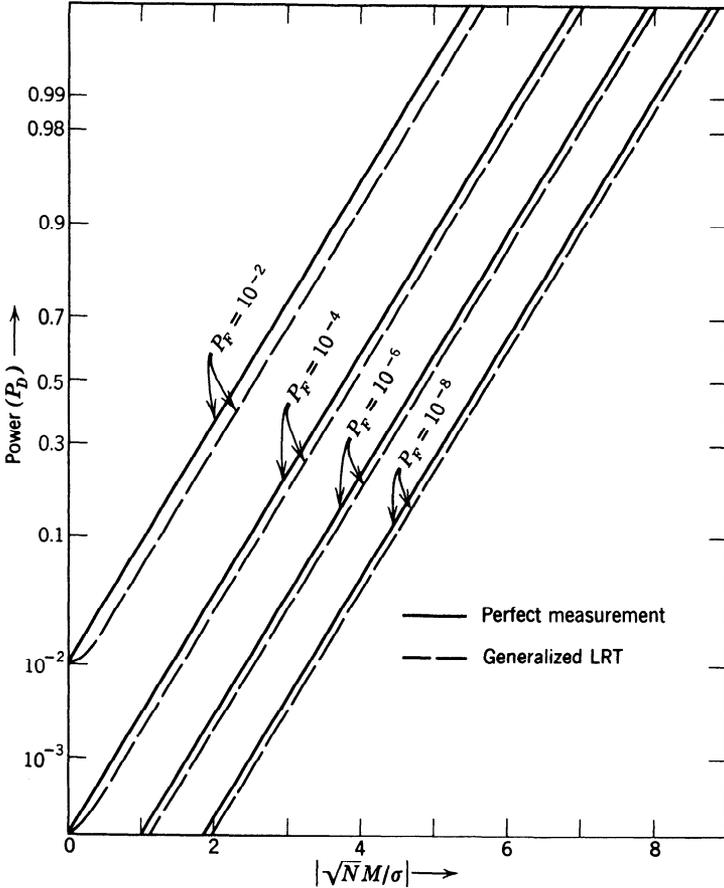
Fig. 2.31 Power function: generalized likelihood ratio tests.
