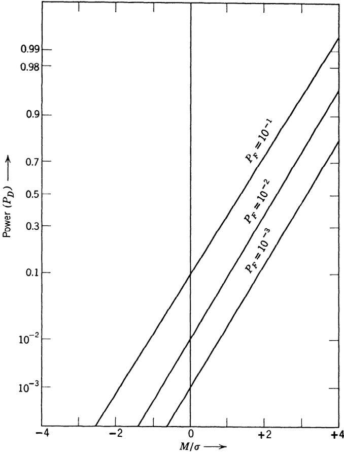
Fig. 2.29 Performance of LRT assuming positive  $M$ .
