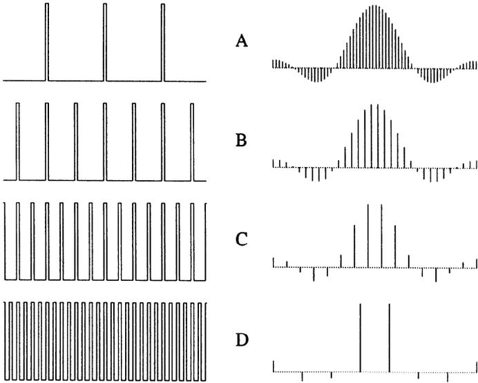
**Figure 3.9:** The effect of changing the period at constant duty cycle. In these figures we see on the left a periodic rectangular signal, and on the right the absolute squares of its FS amplitudes represented as vertical bars placed at the appropriate frequencies. As we progress from (A) through (D) the period is halved each time. Note that as the period is decreased with constant pulse width the frequency resolution decreases but the underlying sinc is unchanged.
