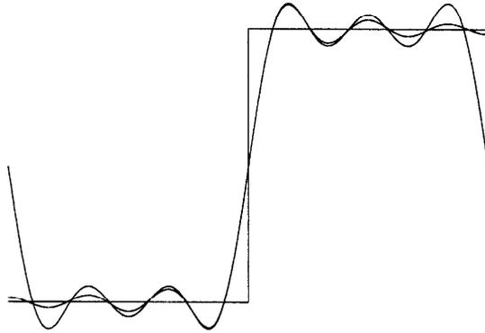
**Figure 3.6:** Gibbs phenomenon for the discontinuity of the square wave at  $t = 0$ . Plotted are the square wave, the partial sum with  $K = 3$  terms, and the approximation using the sine integral.
