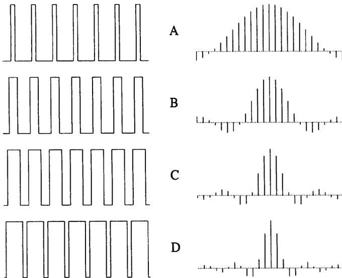
**Figure 3.8:** The effect of changing the duty cycle at constant period. In these figures we see on the left a periodic rectangular signal, and on the right the absolute squares of its FS amplitudes represented as vertical bars placed at the appropriate frequencies. (A) represents a duty cycle of 20%, (B) 40%, (C) 60% and (D) 80%. Note that when the duty cycle vanishes all amplitudes become equal, while when the signal becomes a constant, only the DC term remains.
