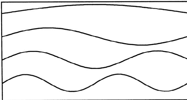
**Figure 3.3:** The instantaneous deflection of a vibrating string may be sinusoidal, and the boundary conditions restrict the possible frequencies of these sines. The top string contains only half of its wavelength between the string's supports; the next contains a full wavelength, the third three-quarters, etc.
