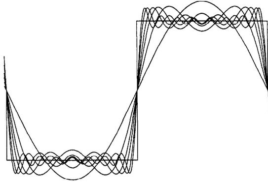
**Figure 3.5:** Partial sums of the Fourier series of a periodic square wave signal  $\square(t)$  for  $K = 0, 1, 2, 3, 5$  and  $7$ . Note that although far from the discontinuity the series converges to the square wave, near it the overshoot remains.
