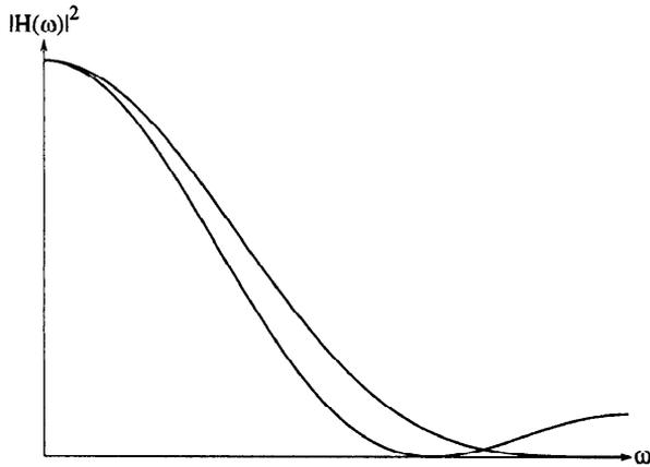
**Figure 6.6:** The (squared) frequency responses of two simple three-point average filters. Both responses are clearly low-pass but not ideal. The average with coefficients goes to zero at  $\frac{1}{2}f_s$ , but is 'wider' than the simple average.
