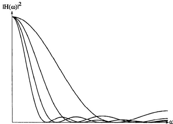
**Figure 6.7:** The (squared) frequency responses of simple averaging filters for  $L = 3, 5, 7$  and  $9$ . We see that as  $L$  increases the pass-band becomes narrower, but oscillations continue.
