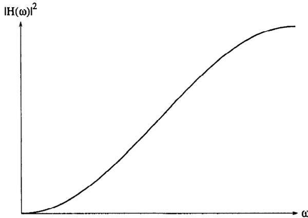
**Figure 6.9:** The (squared) frequency response of a finite difference filter. With these coefficients the lower frequency components are passed essentially unattenuated, while the higher components are strongly attenuated.
