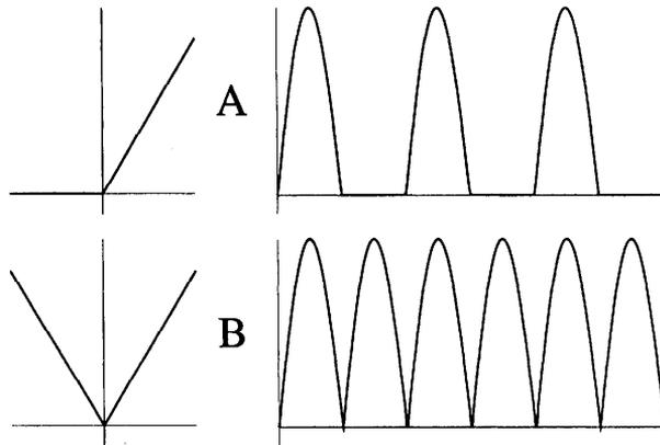
**Figure 6.2:** Half-wave and full-wave rectifiers. (A) depicts the output as a function of input of a half-wave rectifier, as well as its effect on a sinusoid. (B) depicts the same for a full-wave rectifier.
