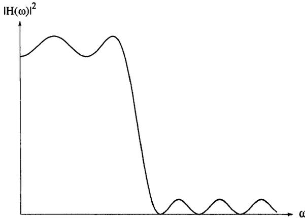
**Figure 6.8:** The (squared) frequency responses of a 16-coefficient low-pass filter. With these coefficients the lower frequency components are passed essentially unattenuated, while the higher components are strongly attenuated.
