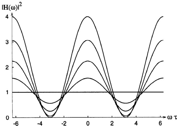
**Figure 6.4:** Amplitude of the frequency response for the echo system with positive coefficients. The amplitude is plotted as a function of  $\omega\tau$ . The coefficients are  $h = 0$  (the straight line), 0.25, 0.5, 0.75, and 1.0 (the plot with zeros).
