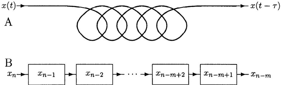
**Figure 6.3:** Implementation of the simple delay. In (A) we see how an analog delay of lag  $\tau$  can be obtained by allowing a voltage or current signal to travel at finite velocity through a sufficiently long delay line. In (B) a digital delay of lag  $m$  is implemented using a FIFO buffer.
