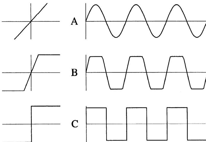
**Figure 6.1:** The effect of clipping amplifiers with different gains on sinusoidal signals. In (A) there is no clipping, in (B) intermediate gain and clipping, while (C) represents the infinite gain case (hard limiter).
