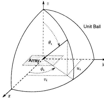
FIGURE 63.4: Definitions of azimuth ( $-180^\circ < \phi_i \leq 180^\circ$ ) and elevation ( $0^\circ \leq \theta_i \leq 90^\circ$ ). The direction cosines  $u_i$  and  $v_i$  are the rectangular coordinates of the projection of the corresponding point on the unit ball onto the equatorial plane.
