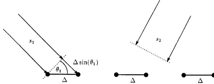
FIGURE 63.1: Planar array composed of  $m = 3$  pairwise identical, but displaced, sensors (doublets).
