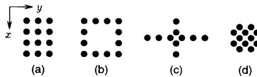
FIGURE 63.9: Centro-symmetric array configurations with a dual invariance structure: (a) URA with  $M = 12$ ,  $m_x = 9$ ,  $m_y = 8$ . (b) URFA with  $M = 12$ ,  $m_x = m_y = 6$ . (c) Cross array with  $M = 10$ ,  $m_x = 3$ ,  $m_y = 5$ . (d)  $M = 12$ ,  $m_x = m_y = 7$ .
