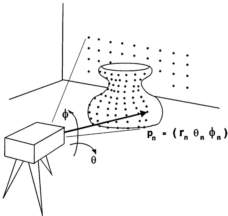
**FIGURE 9.4** Range images are typically an array of individual range values sampled while changing the pointing direction (e.g., azimuth and elevation angles) of a ranging device. A digital range image of the polar form shown can be readily transformed into rectangular coordinates if required.
