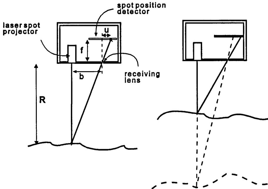
**FIGURE 9.5** A simple pinhole camera model illustrates the basic active triangulation principle. As the distance  $R$  to the target surface changes, the spot position  $u$  on the detector changes, maintaining similarity between the large triangle outside the camera and the small triangle inside. There is an inverse relationship between  $R$  and  $u$ .
