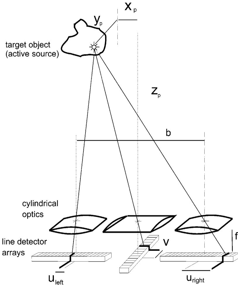
**FIGURE 9.8** The OPTOTRAK position tracking system employs a novel arrangement of cylindrical optics and one-dimensional detectors to triangulate the 3-D position of an infrared LED target. Up to 255 individual multiplexed targets can be tracked by the system.
