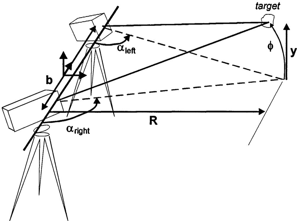
**FIGURE 9.2** The basic triangulation geometry as used in classical surveying determines the distance to a remote point by sighting it from two locations separated by a known baseline. The pointing angles  $\alpha_{\text{left}}$  and  $\alpha_{\text{right}}$  are measured locally.
