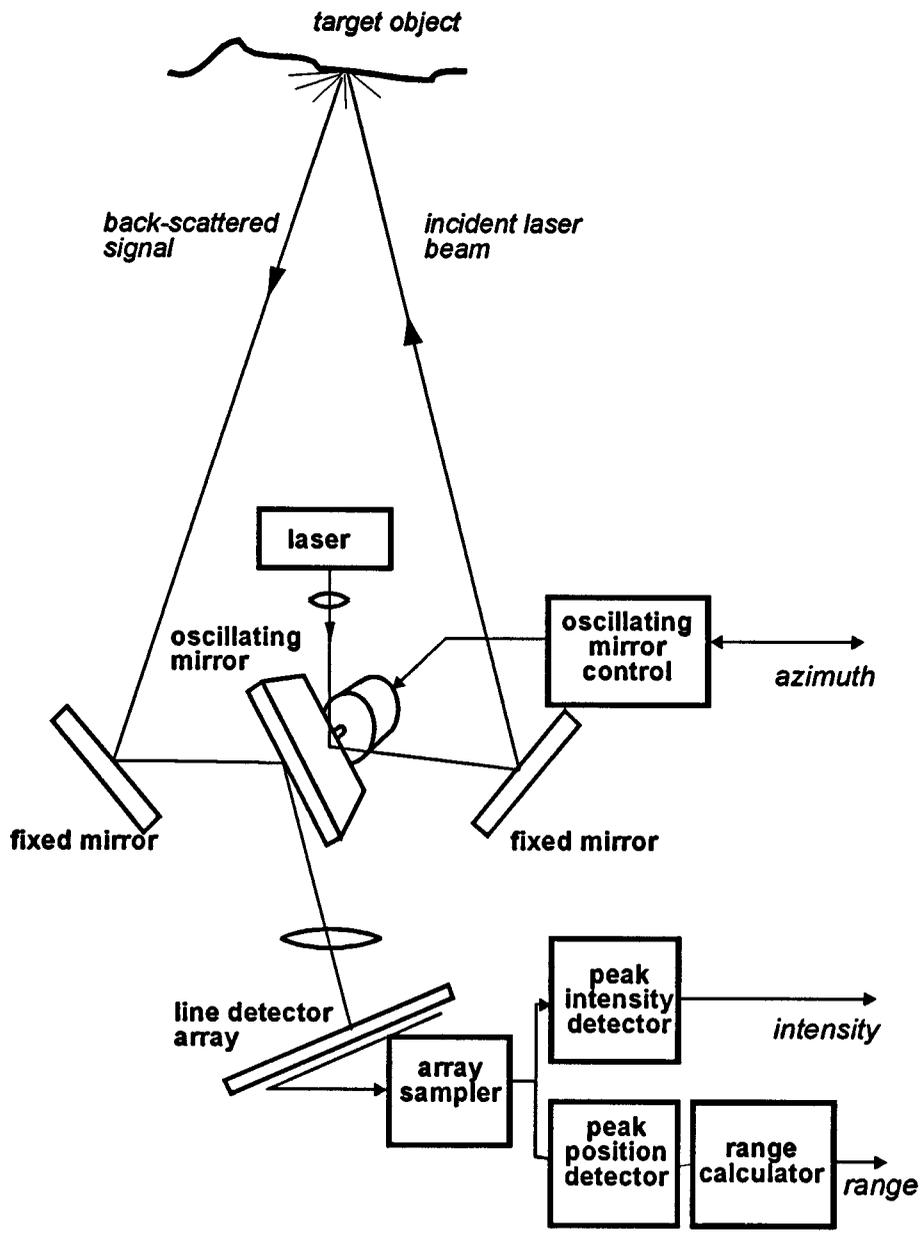
**FIGURE 9.6** The Hymarc laser triangulation line scanner uses the synchronized scanning principle. Both sides of an oscillating mirror are used to sweep both the projected beam and the axis of detection over the target. The detector array is tilted to the lens plane to maximize the depth of focus.
