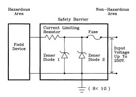
**FIGURE 100.1** Major components of barrier circuit.
