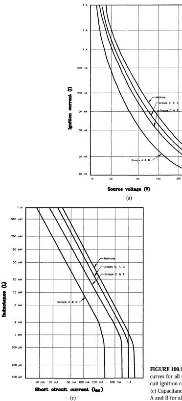
**FIGURE 100.2** (a) Resistance circuit ignition curves for all circuit metals. (b) Inductance circuit ignition curves at 24 V for all circuit metals. (c) Capacitance circuit ignition curves for groups A and B for all circuit metals.
