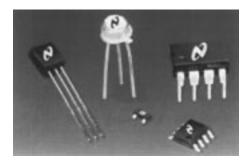
FIGURE 32.47 Plastic TO-92, TO-99 metal can, 8-lead DIP, 8-lead SOIC, and TinyPak<sup>™</sup> SOT-23 plastic packages. (Courtesy National Semiconductor Corp.)
