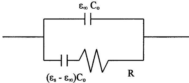
FIGURE 46.3 Equivalent circuit of a parallel-plate capacitor based on the Debye model.
