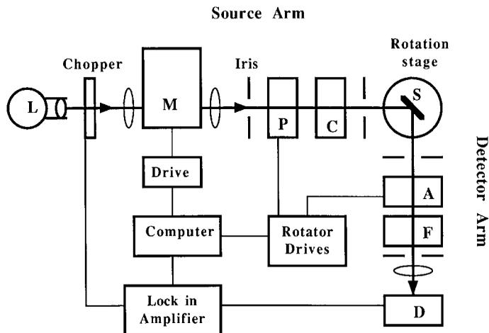
**FIGURE 60.7** Schematic diagram of a PCSA reflection null ellipsometer, which is composed of five systems: the source system, polarimetric system, sample system, detection system, and computer system. The symbols are L = light source, M = monochromator, F = wavelength filter, and D detector. The symbols P, C, S, and A have their customary meanings.
