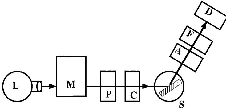
FIGURE 60.6 Schematic diagram of a PCSA ellipsometer.
