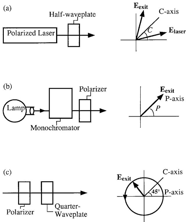
**FIGURE 60.5** Generation of light linearly polarized at a desired direction using (a) a laser source and a half-wave plate and (b) a lamp, monochromator, and a polarizer, plus (c) generation of circularly polarized light using a polarizer and a quarter-wave plate.
