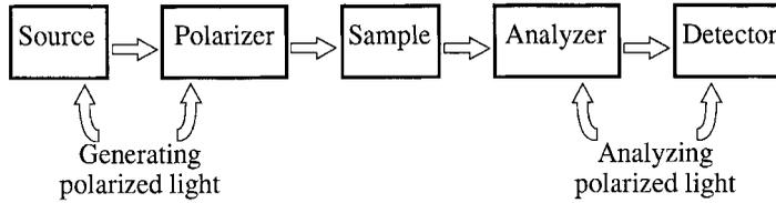
**FIGURE 60.4** Schematic diagram of a polarimeter to measure polarization response. The light source and polarizer are used to generate polarized light, and the analyzer and detector are used to analyze the state of polarization of the light.
