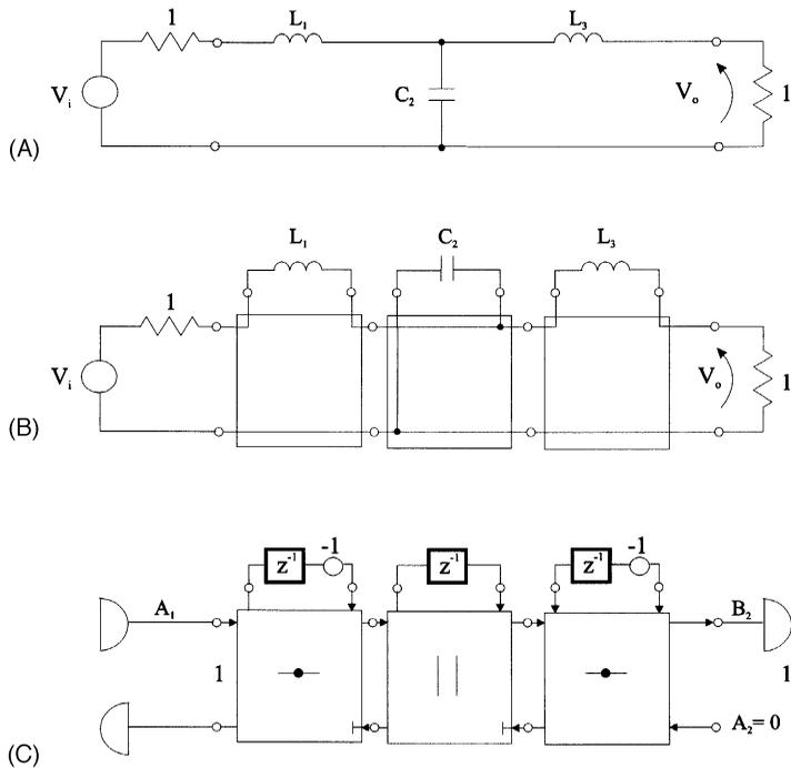
**FIGURE 82.15** Digital wave filters establish equivalence with classical filter circuits by use of wave adaptor substitutions: (A) *LC* reference low-pass; (B) identification of wire interconnections; (C) corresponding wave digital filter.
