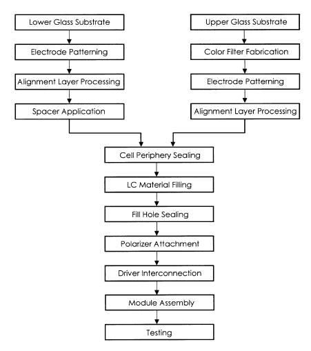
FIGURE 92.9 LCD assembly flowchart.
