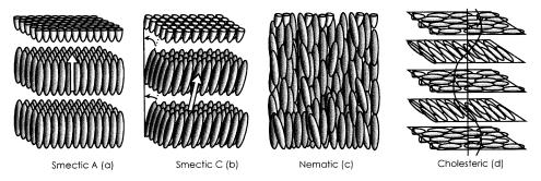
FIGURE 92.2 Molecular orientation in (a) smectic A, (b) smectic C, (c) nematic, and (d) cholesteric LC phases.
