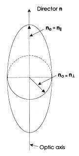
**FIGURE 92.5** Refractive index anisotropy of uniaxial LC.
