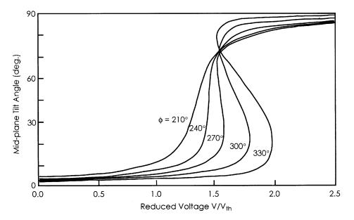
**FIGURE 92.11** Calculated curves of tilt angle of local directors in the midplane of an STN cell as a function of reduced voltage  $V/V_{\text{th}}$ , where  $V_{\text{th}}$  is the Freedericksz threshold voltage of a nontwisted layer with a zero pretilt angle. The steepness of the curves increase as the twist angle,  $\Phi$ , is increased, and bistability is achieved when  $\Phi > 240^\circ$ .
