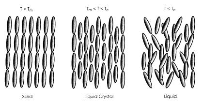
**FIGURE 92.1** Illustration of a solid, an LC, and a liquid. A solid has an orientational as well as a positional order for the molecules. An LC has an orientational order only. A liquid phase is isotropic with neither positional nor orientational order.
