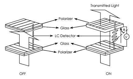
**FIGURE 92.12** Illustration of an ECB display: (a) with homeotropic alignment and crossed polarizers, the off-state is black; (b) in the on-state, the output light through the LC is elliptically polarized due to the LC birefringence and the light is transmitted through the crossed polarizer.
