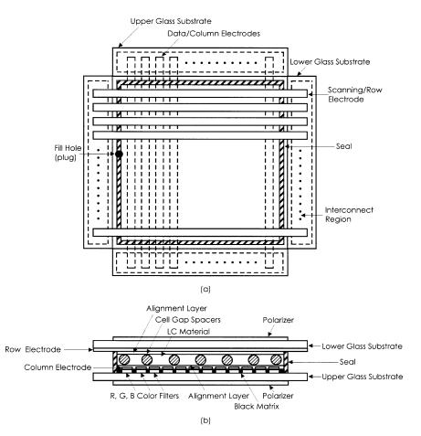
FIGURE 92.8 Plan (a) and cross-sectional view (b) of a passive matrix-addressed LCD.
