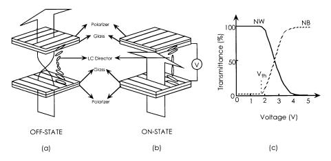
**FIGURE 92.10** Illustration of TN effect: (a) in the off-state, the incident polarized light is transmitted through the entrance polarizer, the 90° TN LC, and the crossed exit polarizer; (b) in the on-state; (c) the solid line shows the voltage-transmission behavior for the NW configuration, shown in (a) and (b), with crossed polarizers. The dashed line is for an NB configuration with parallel polarizers.
