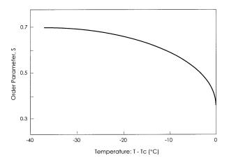
**FIGURE 92.3** Temperature dependence of the order parameter *S* of the nematic LC *P* = azoxy anisole (PPA) [10]. *S* decreases with increasing temperature *T*, and rapidly approaches 0 near the clearing temperature,  $T_c$ .
