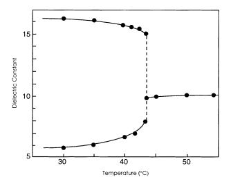
**FIGURE 92.4** Temperature dependence of dielectric constant of the nematic LC cyanobiphenyl at a frequency of 100 KHz [13] exhibiting positive dielectric anisotropy ( $\varepsilon_{\parallel} > \varepsilon_{\perp}$ ).  $\varepsilon_{\parallel}$  decreases with temperature, whereas  $\varepsilon_{\perp}$  increases with temperature until both are equal at the clearing temperature corresponding to the isotropic liquid.
