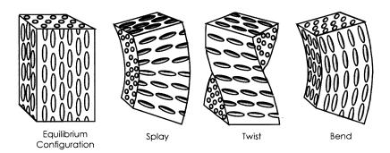
**FIGURE 92.7** Deformation of nematic LC molecules from equilibrium configuration is shown in (a). Three types of deformations — (b) splay, (c) twist, and (d) bend can describe all possible types of deformations.
