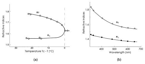
**FIGURE 92.6** (a) Temperature dependence of the refractive indices  $n_{\parallel}$  and  $n_{\perp}$  for a nematic LC MBBA at  $\lambda = 546$  nm; (b) wavelength dependence of refractive indices of the nematic LC 4-butoxyphenyl ester of 4'-hexyloxybenzoic acid at 80°C.
