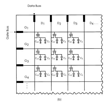
**FIGURE 92.13** (a) AM LCD module electronics block diagram; (b) magnified view of the region shown in (a) illustrating active matrix TFT array.
