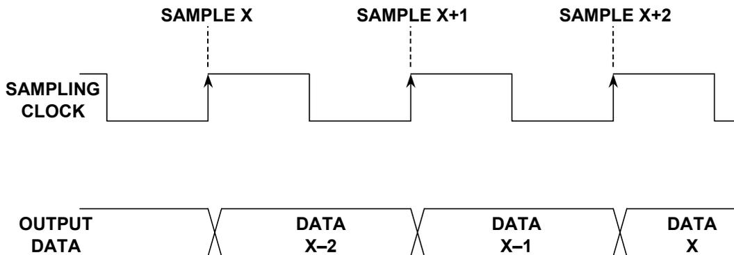
ABOVE SHOWS TWO CLOCK-CYCLES PIPELINE DELAY
