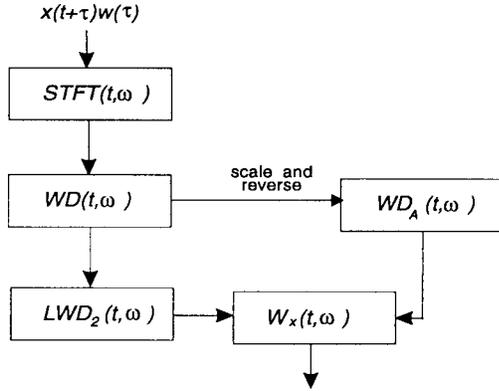
Fig. 1. Block schema for the PWVD realization.
