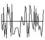
Figure 14: One waveform period stored in wavetable.
