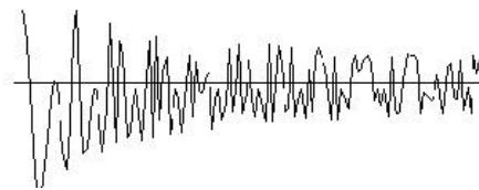
Figure 16 : Repeated waveform modulated by an amplitude envelop.
