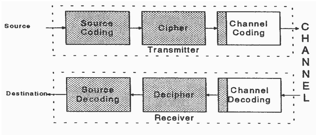
A standard module (Rockwell Socket-Modem) is used for channel coding over the PSTN. Modem functions are well suited for DSP-based implementation.<sup>10</sup>
