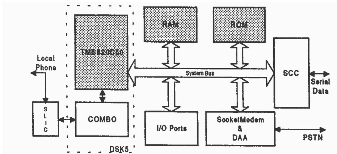
To support facsimile group 3 ciphering, this system is designed to incorporate an extra Socket-Modem. Fax machines with a digital interface are linked to the serial port.
