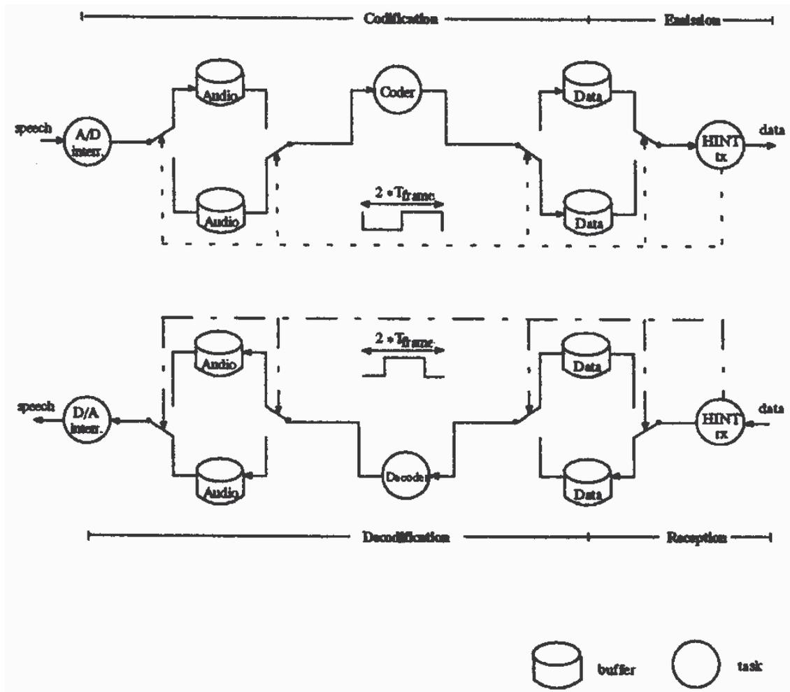
This computational model has two main background processes (Coder and Decoder) and several foreground tasks associated with hardware interrupts. Foreground tasks virtualize an input/output block system. The transmitter works this way: in the codification process one block of speech samples (Audio buffer) is transformed into one encrypted data frame while the emission sends another data frame (Data buffer). The data frame includes synchronization and error control information.
