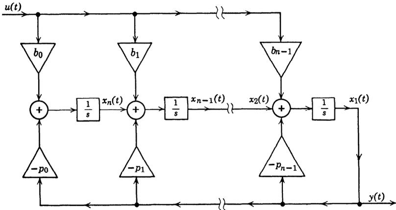
Fig. 6.30 Canonic realization No. 2: state variables.
