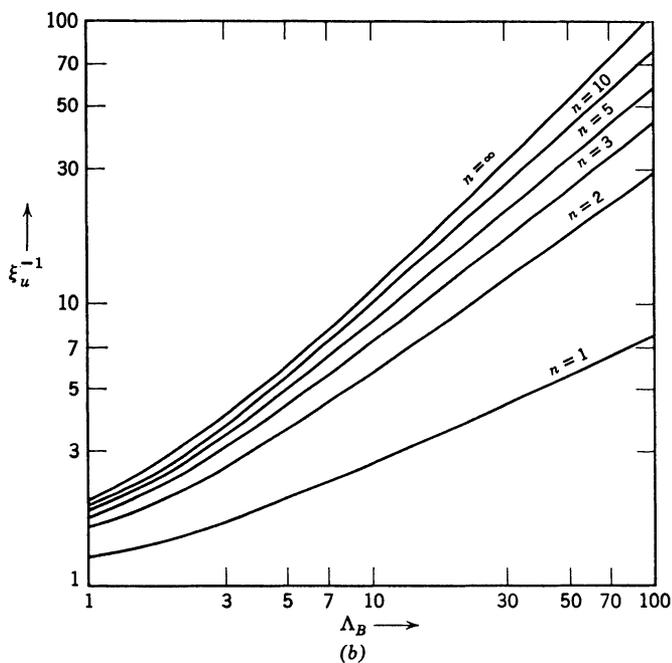
Fig. 6.17 Reciprocal of mean-square error, Butterworth spectra: (a) realizable; (b) unrealizable
