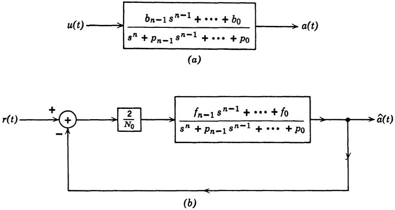
Fig. 6.21 Filters: (a) message generation; (b) canonic feedback filter.
