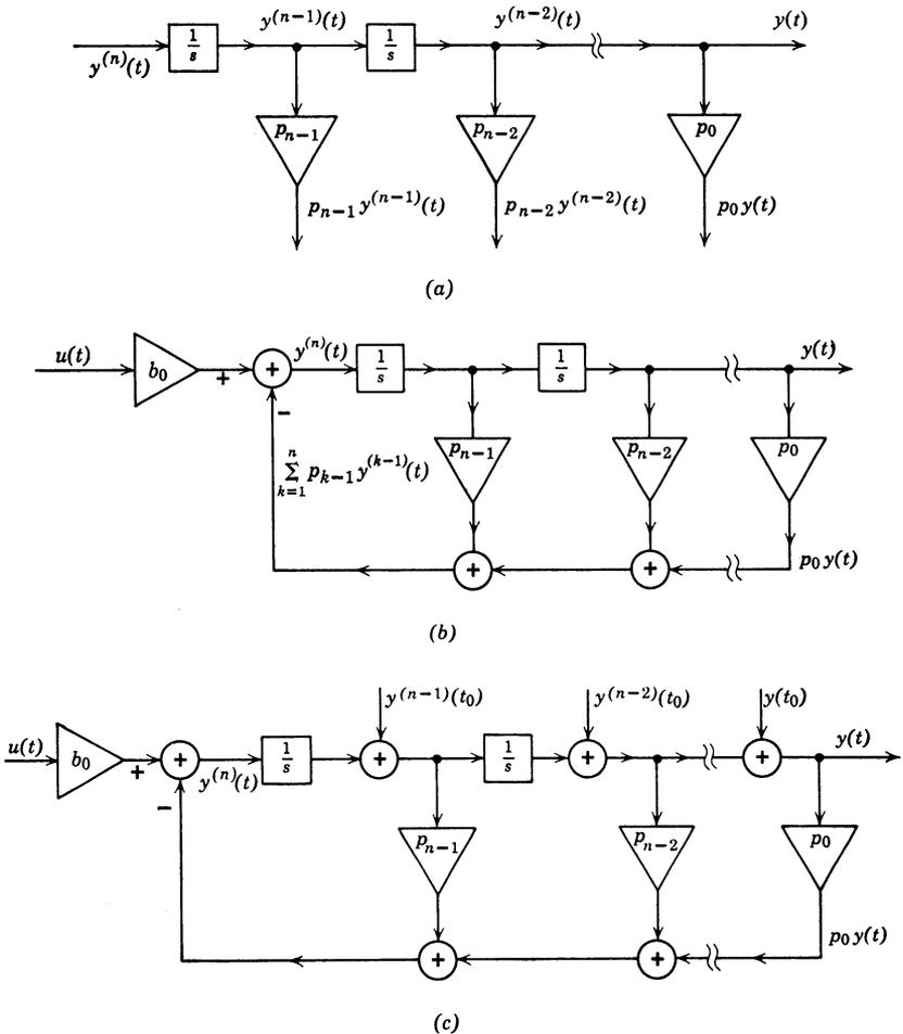
Fig. 6.27 Analog computer realization.
