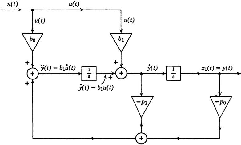
Fig. 6.28 Analog realization.
