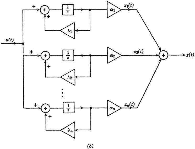
Fig. 6.31 Canonic realization No. 3: (a) transfer function; (b) analog computer realization.
