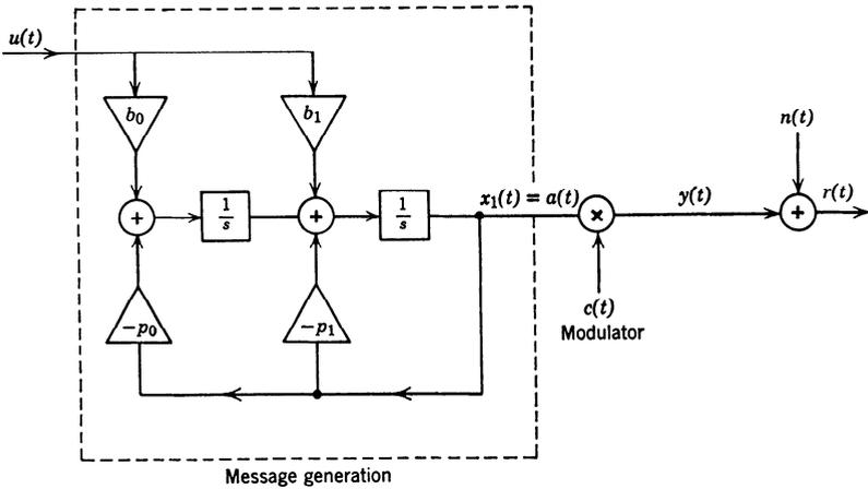
Fig. 6.34 A simple case of linear modulation in the state-variable formulation.
