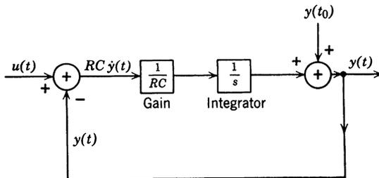
Fig. 6.26 An analog computer realization.
