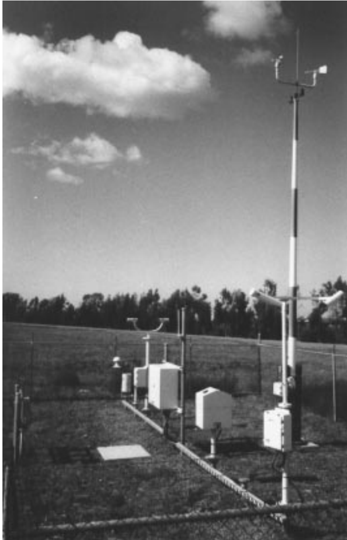
FIGURE 73.6 A view of an ASOS system sited at an airport near San Diego. The instrument of Figure 73.5 is seen in the foreground. A stand for the freezing rain sensor is not used. The next instrument is the ceilometer. Behind that is a metal box containing connections to the sensors and instruments to transmit the data to a remote collection and processing station. Along the same line of instruments beyond this is the precipitation identification or present weather sensor. This is followed along the same line by the sensor measuring ambient and dewpoint temperatures and a tipping bucket rain gage. To the north of the line of instruments is a pole with a cup anemometer, weather vane, flashing red lights, and lightning rod at the top.
