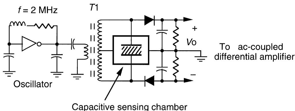
**FIGURE 81.13** FM demodulator technique applied to measurement of the flow of small seeds in an agricultural machine application. The relative permittivity of the seeds causes the resonant frequency of the discriminator circuit to shift and to produce a change in the output voltage. The claimed sensitivity of this circuit is on the order of tens of femtofarads. The cross-hatched region of the sensing chamber represents the active area through which the seeds flow.
