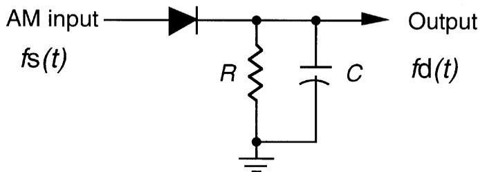
**FIGURE 81.4** Envelope detector for full-carrier AM signals.
