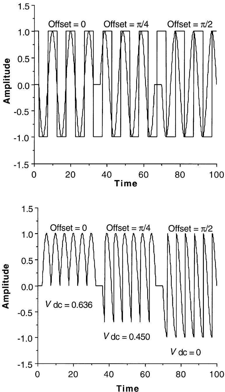
**FIGURE 81.6** Gating of a constant-amplitude sinusoidal by a square wave in a switching phase-sensitive demodulator with various phase offsets between the carrier and the square wave. The upper trace shows the carrier and the square wave; the lower trace shows the signals which appear at the output of the differential amplifier in Figure 81.5 (b). The dc output voltages of the low-pass filter are indicated for each value of phase offset.
