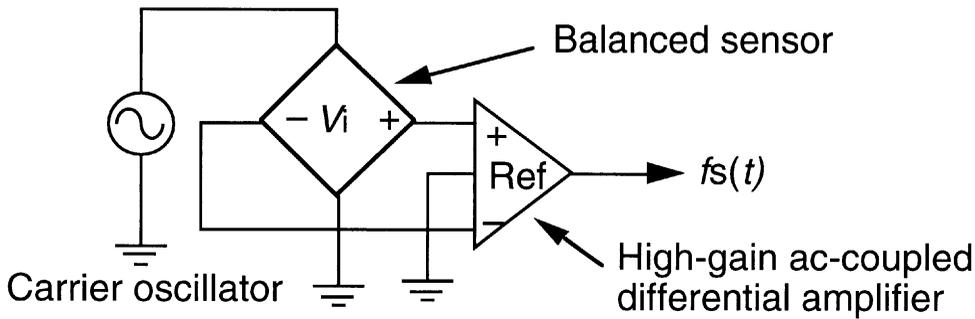
**FIGURE 81.3** A balanced sensor with ac excitation and a differential-amplifier output stage. Typical sensors which might be found in this role are resistive Wheatstone bridges, differential-capacitance pressure sensors or accelerometers, or linear-variable differential transformers (LVDTs). Variation in the sensor measurand produces a DSB suppressed-carrier signal at the amplifier output.
