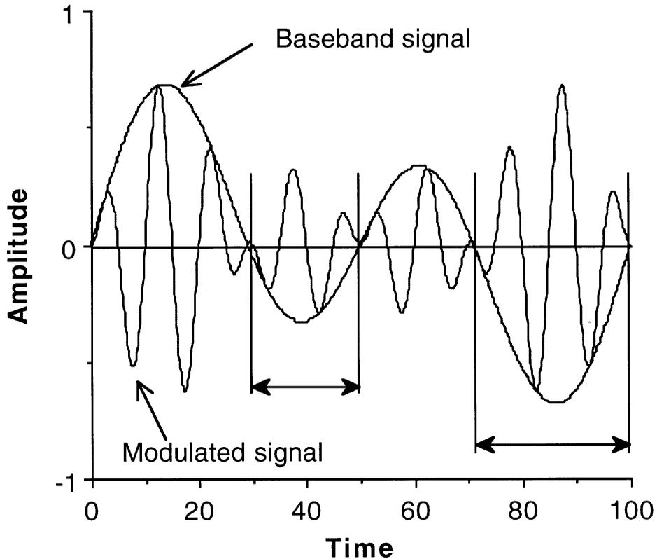
**FIGURE 81.2** Time-domain representation of a DSB suppressed-carrier signal. Regions demarcated by double arrows indicate phase inversion of the modulated signal relative to the unmodulated carrier. This is in contrast to full-carrier AM in which the modulated signal is always in phase with the carrier.
