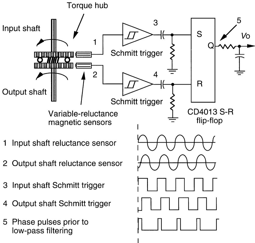
**FIGURE 81.11** Use of phase-sensitive demodulation to measure torque in a rotating shaft as described by Sokol et al. [15]. Typical waveforms and the points in the circuit where they are found are indicated. The  $RC$  coupling to the S and R terminals of the CD4013 flip-flop provides for edge triggering.
