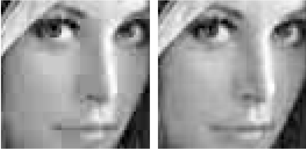
FIGURE 14.5 Zoom of image compressed using JPEG at 0.5 bit per pixel. (a) DCT, (b) LOT.
